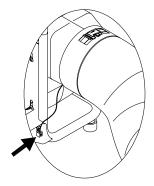
Grounding lug provided for ground wire attachment from conductive duct.
