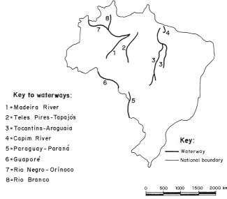
Figure 2 Industrial *hidrovias* (waterways) for soybean transport. Waterways 1, 4 and the southern part of 5 are partially operational; 2 and 3 are in advanced stages of the licensing process; the northern part of 5 is included in Forward Brazil plans, and 6, 7 and 8 are in preliminary stages of discussion.
