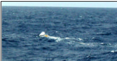
The top float surfing through the waves as it is being dragged down by the anchor falling to the bottom. We chased it, until it disappeared underwater, hopefully not to be seen again until the mooring is recovered in April 2004.
