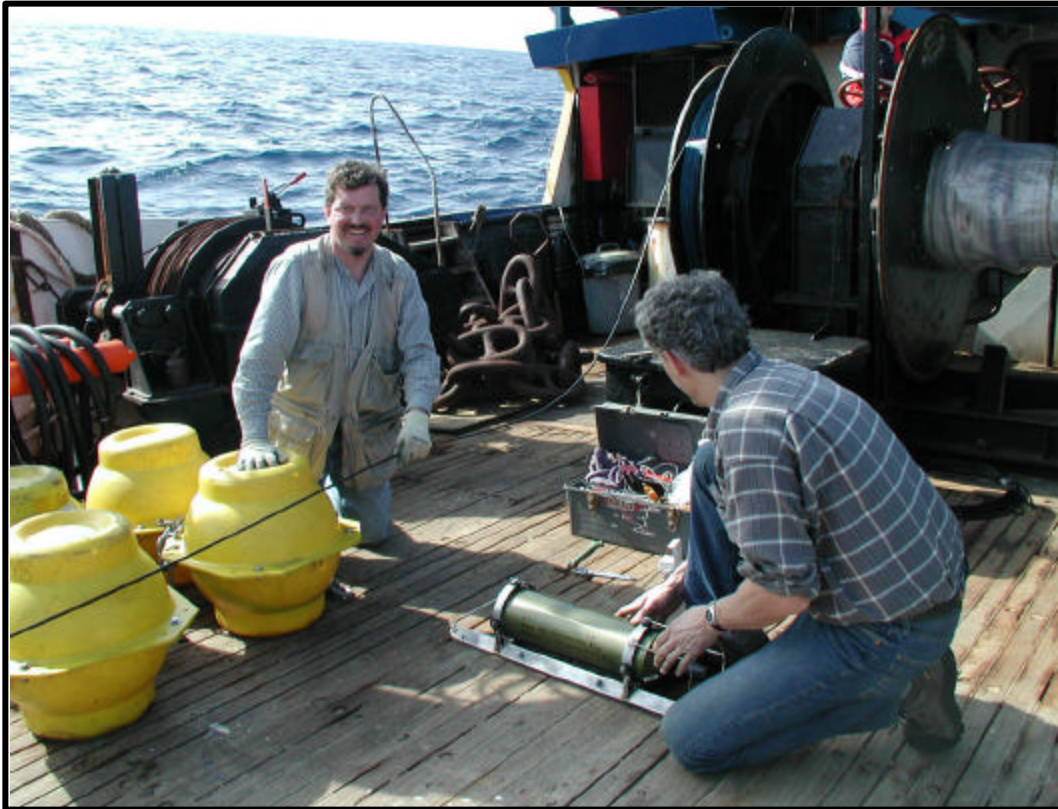
Jeff Nystuen and Eric Boget attaching an Acoustic Rain Gauge (ARG) to the mooring line.
