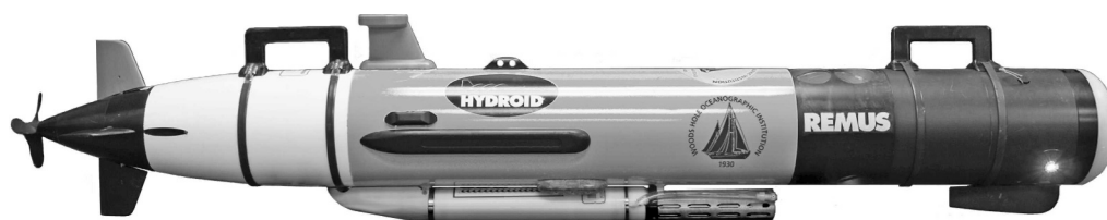
Fig. 2. The customized autonomous underwater vehicle REMUS. Vehicle length is approximately 1.8 m. The vehicle is capable of reaching depths of 90 m. Note the SeaBird 49 CTD attached to the lower portion of the vehicle and the excitation light of the BB2F fluorescence meter.
