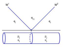
Left-going wave  $\mathcal{W}^1=q_m-q_l$  and right-going wave  $\mathcal{W}^2=q_r-q_m$  are eigenvectors of A.
