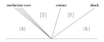
Solution is constant on any ray: q(x,t) = Q(x/t) A "similarity solution".
