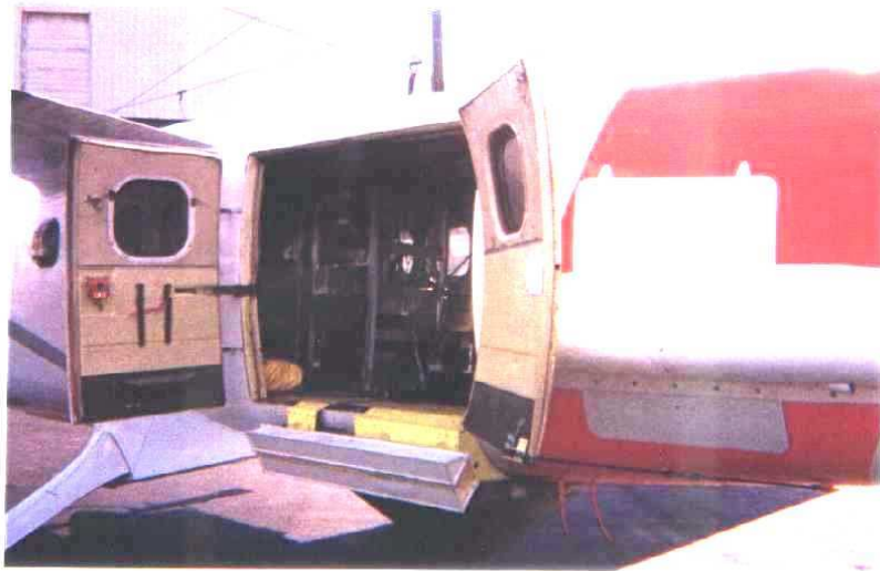
Figure 1: The COherent Real Aperture Radar, CORAR, mounted on the CIRPAS Twin Otter aircraft. The white 120 cm slotted waveguide antennas below the door are the fixed, side-looking antennas. Two, back-to-back, 45 cm long, slotted waveguide antennas are mounted on a stabilized, rotating mount inside the gray radome beneath the fuselage, directly behind the sidelooking antennas in these pictures.
