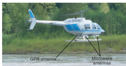
Figure 1. The helicopter at the Cowlitz River. Two microwave antennas are located just below the cabin on each side. The GPR antenna is the large white structure below the helicopter.
