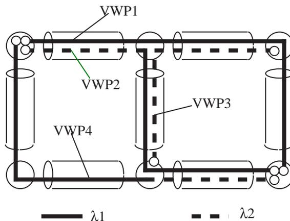
Figure 3: Virtual-wavelength-path routing in a small example network (after [12])
