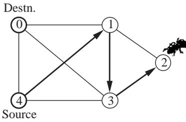
Figure 4: Ant at a dead end (node 2) *en route* from node 4 (source) to node 0 (destination)
