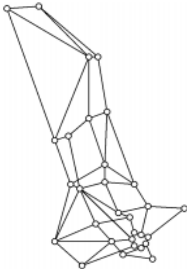
FIGURE 1. This network topology is the same as the interconnection structure of the Synchronous Digital Hierarchy network of British Telecom, and provides a realistic network topology
