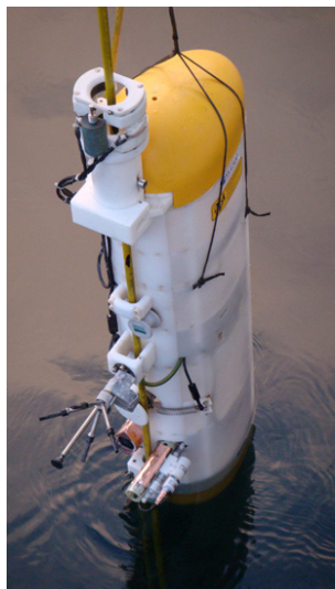
Figure 3: The McLane moored profiler (MMP) modified with an inductive power coupler.
