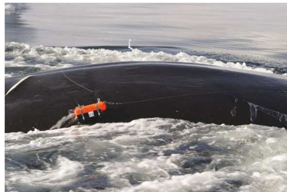
Figure 2. Instrument attached to bowhead whales with 1.5-m long wire and small harpoon head imbedded in the blubber layer. A WetLabs FLNTUB fluorometer was fixed to a float using hose clamps. Flotation (orange float) kept the tag at the surface for instrument recovery after the package was released from the whale, and the tag was relocated using a satellite (top left of orange float) and VHF transmitter (top right of orange float). The package corroded off the whale after 24–48 h using a magnesium bolt. Photo by M. P. Heide-Jørgensen.
