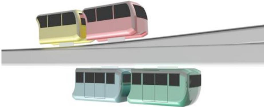
Coupled operation. Coupled operation is where two podcars are virtually linked (they run bumper to bumper) and are only allowed to split up at diverge points where each vehicle leader and follower has its own track and so no possibility of energetic collision. Merging is done at bumper speed typically in stations.
