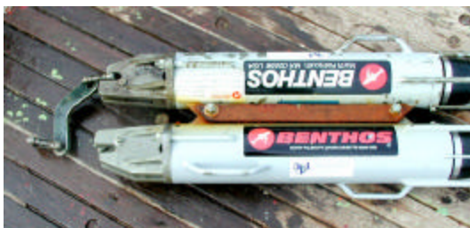
The acoustic releases. The one on the bottom has “released” the metal bar, which held the line to the anchor, on the left.
