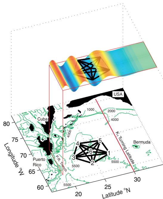
**Figure 5.** The AMODE acoustic tomography array detected diurnal tidal signals ( $K_1$  and  $O_1$  frequencies) of the lowest internal wave mode. The predicted horizontal variation of the displacement associated with this mode for the  $K_1$  frequency is shown at the top as the coloured wave. The southern boundary is the 600-km long shelf just north of Puerto Rico (From Dushaw and Worcester, 1998).
