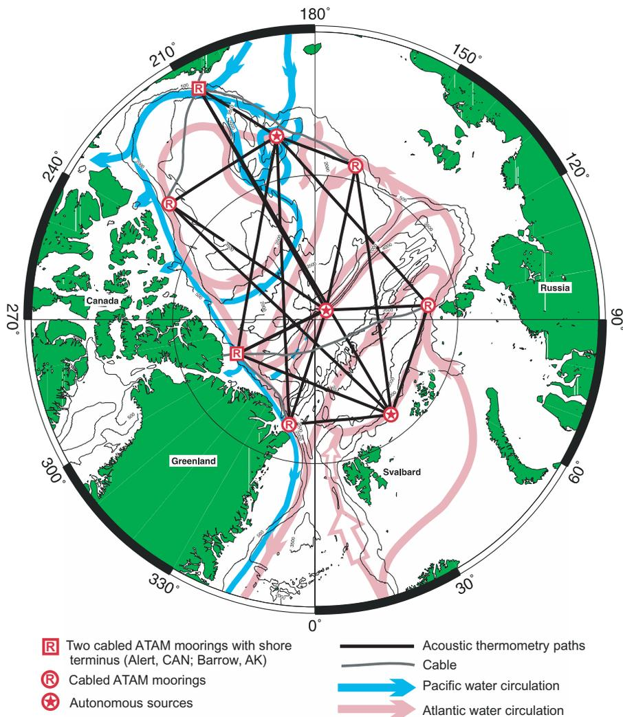
**Figure 14.** A future notional monitoring grid in the Arctic Ocean exploiting synoptic acoustic remote sensing with *in situ* measurements cabled to shore at Alert, Canada (where an existing slant-drilled sea-shore interface already exists), and Barrow, Alaska. ATAM, acoustic thermometry and autonomous monitoring. The Arctic Ocean circulation is taken from McLaughlin et al. (1996).
