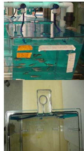
Figure 6.1 A) Aquatic habitat tank with adult baffle properly installed. B) AH tank properly installed on fish rack.
