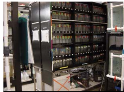
Figure 4.1 Zebra fish modular system used for juvenile fish rearing
