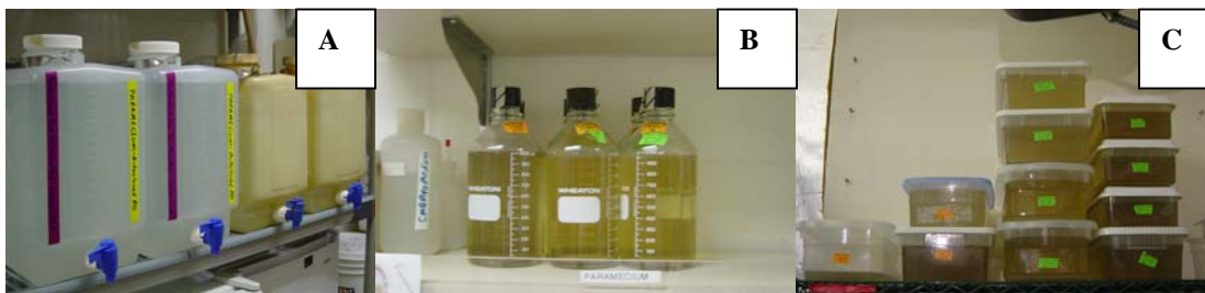
Figure 4.5 A. Autoclaved R.O. water in carboys. B. Paramecium bottle culture. C. Tub culture.
