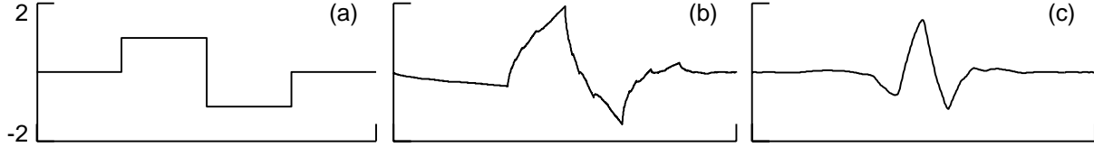
Figure 3. Three mother wavelets: (a) the Haar wavelet; (b) Daubechies's D_4 wavelet (Strang, 1989); (c) Daubechies's least asymmetric wavelet of order 8 (Daubechies, 1992).
