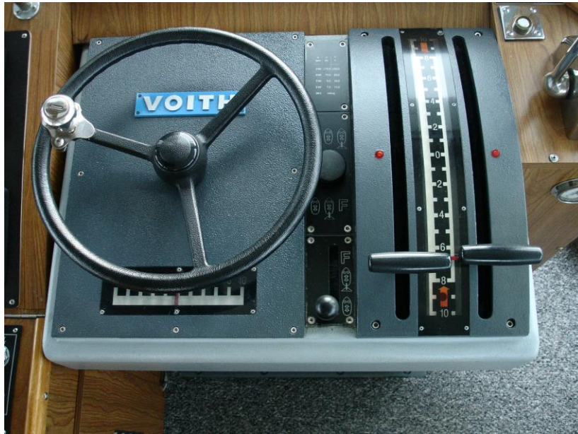
Figure 47: Direction and pitch controls in the pilothouse of the Garth Foss
